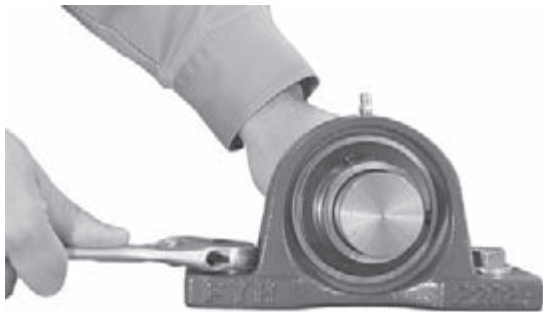
Fig. 14.4 Installation of setscrew units
