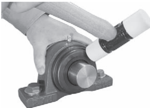
Fig. 14.13 Installing steel plate covers
