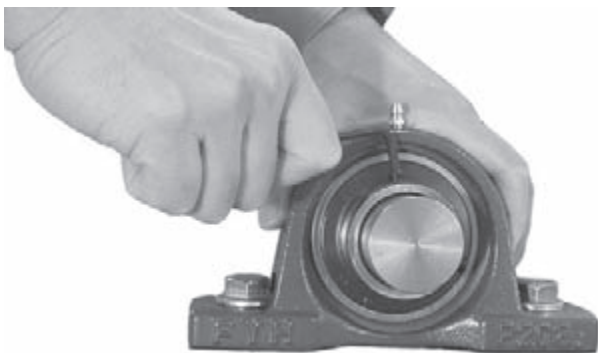
Fig. 14.5 Tightening of set screws
