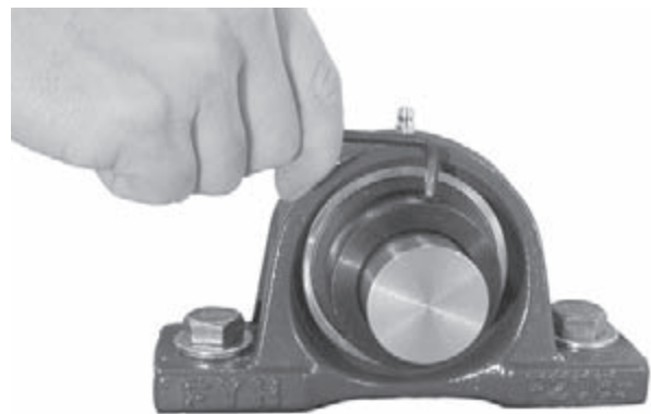
Fig. 14.10 Installing eccentric locking collar
